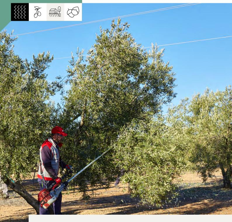
The **SC904R** shaker for olive harvesting and other fruits is an ergonomic and lightweight machine with excellent performance even for professional use. The combination of elements such as low weight, the handle with anti-vibration system, padded leg protection and powerful motor designed for shakers allow efficient and fast collection work.
