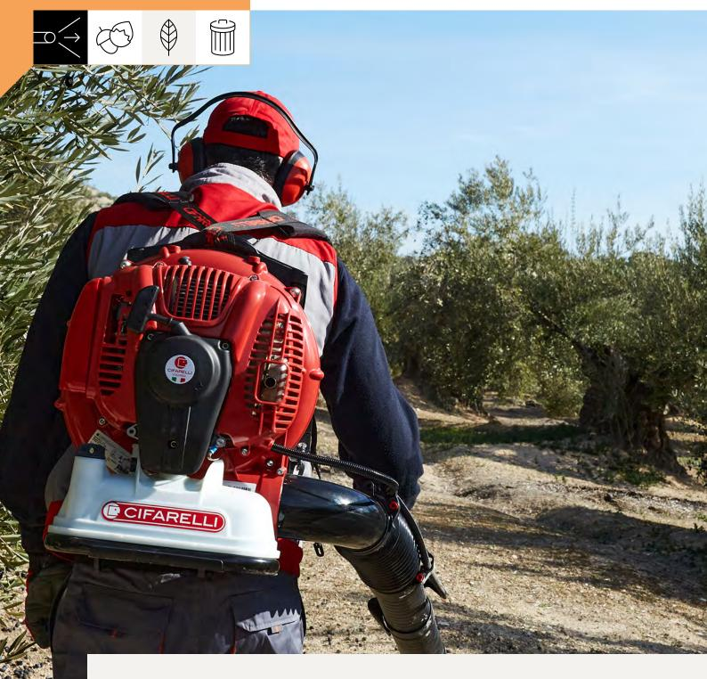
The new **BL2200** blower combines the power of the two-stroke Cifarelli C7 engine with an even more compact design. The machine has a side air filter and a new shoulder support system which makes it less bulky in height than the BL1200. The new design makes this blower even more manageable and allows you to work even in narrow areas and under the plants without the branches fitting into the filter.
